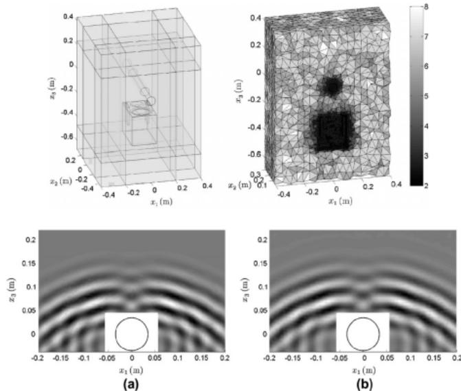
Figure: Snapshots of (a) simulated and (b) measured reasure field.
