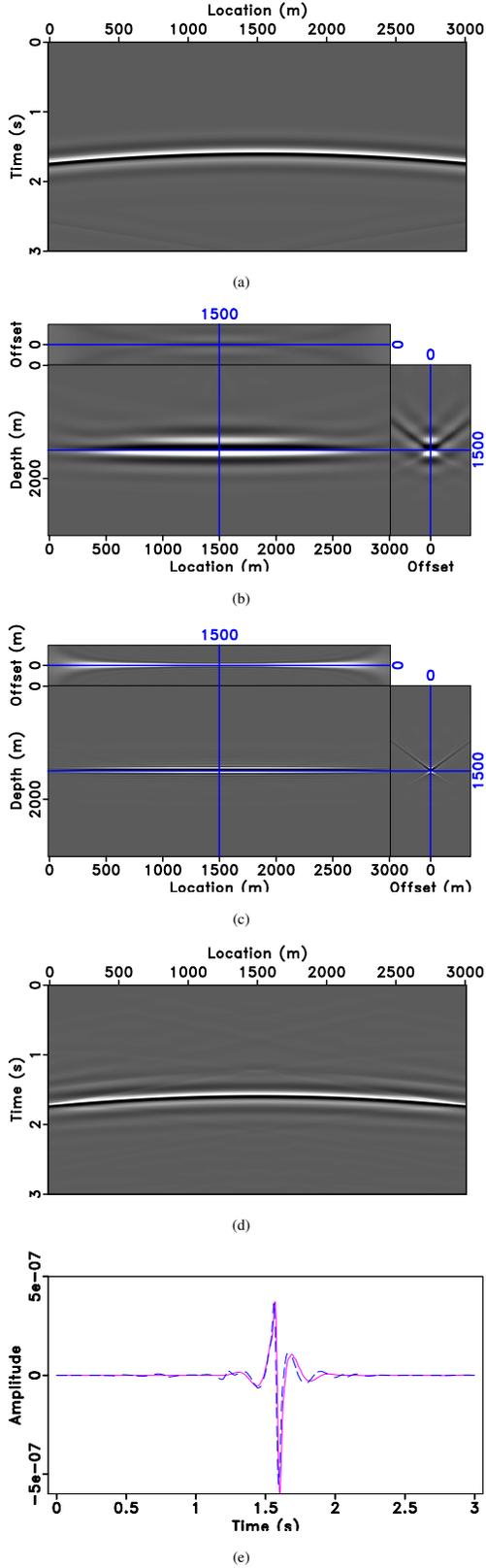
Figure 1: (a) One-shot ( $x_s = 1500m$ ) Simulated Born Data (b) Extended RTM image (c) Inverted Image (d) Resimulated Data of the Inverted Image (e) One trace comparison ( $x = 1500m$ ) between the observed data (red solid line) and predicted data from inverted image (blue dashed line)
