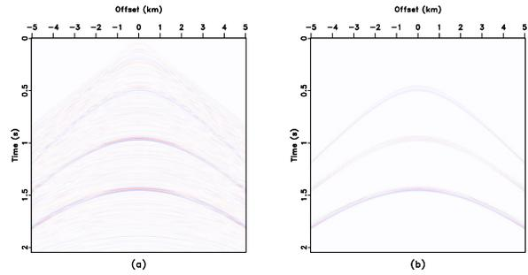
Figure 6: Residual with (a) CGG method; (b) DGAN method
