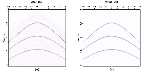
Figure 5: Reconstructed data with (a) CGG method; (b) DGAN method
