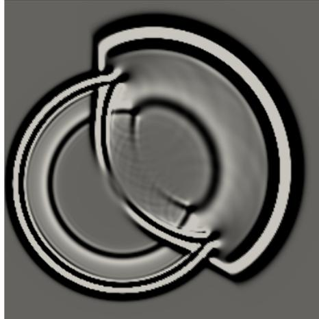
**Figure 6.5:**  $Q_1$  FEM solution snapshot at  $T = 0.75$  s on the dipping model, regular grid quadrature for mass and stiffness matrices.
