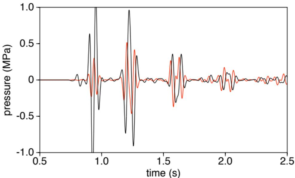
Trace 100 (offset 280 m) for  $\Delta x = 5\text{m}$  (black) vs. error estimated from  $\Delta x = 5\text{m}, 10\text{m}$  (red). Note that after 1.5 s, error appears to be 100%!
