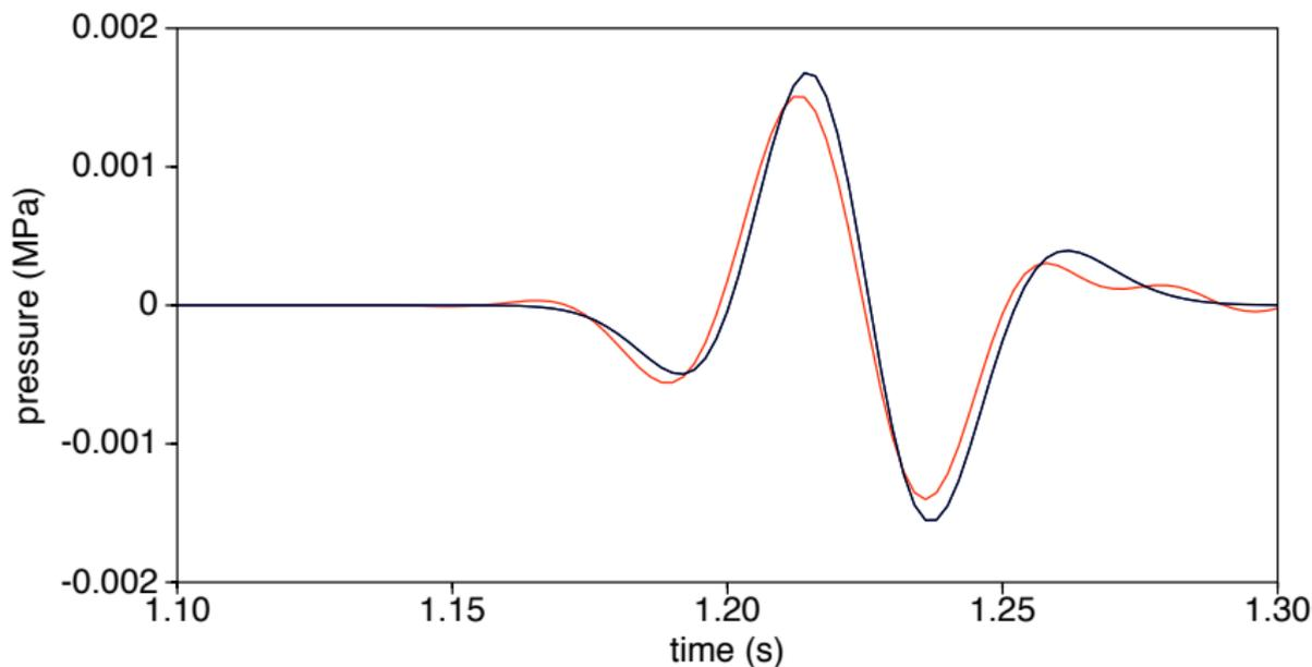
**Homogeneous case!** Trace 100 (offset 280 m),  $\Delta x = 5\text{m}$  (black), 10m (blue), 20m (red)
