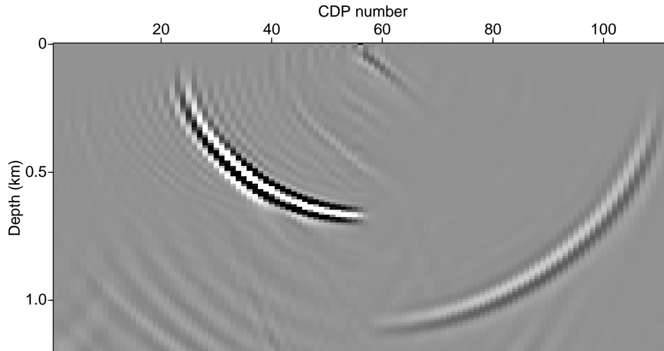
Vertical slice through the migrated cube of an impulse response in a two-velocity medium. The operator used is a 25-point WLSQ operator, along with the Hale-McClellan transform.
