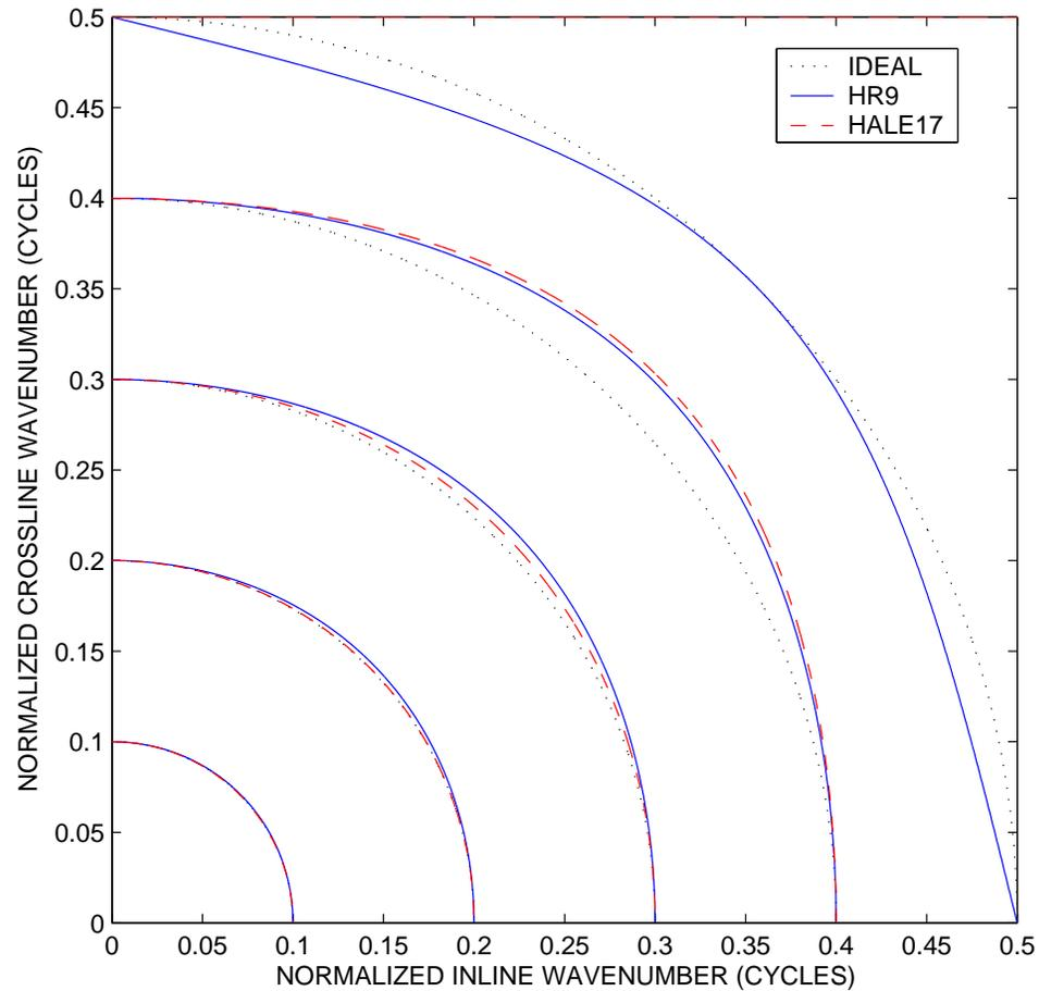
Contours of constant amplitude and phase (constant  $|\mathbf{k}|$ ) for the (scaled and shifted) Hazra & Reddy transformation compared to the improved McClellan transformation.
