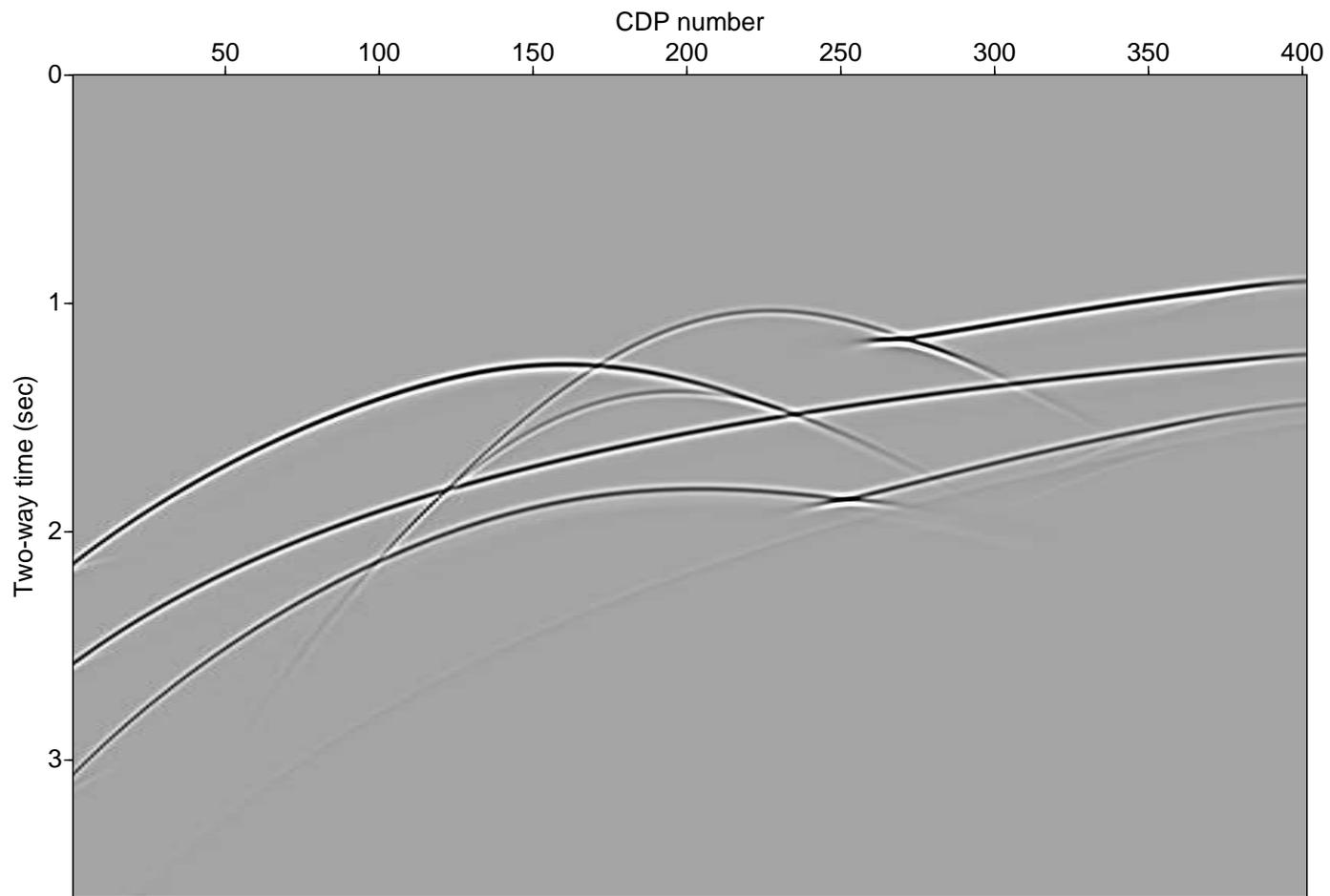
Synthetic data created with 101 cross-lines spaced 40m apart, and 401 in-lines spaced 25m apart.
