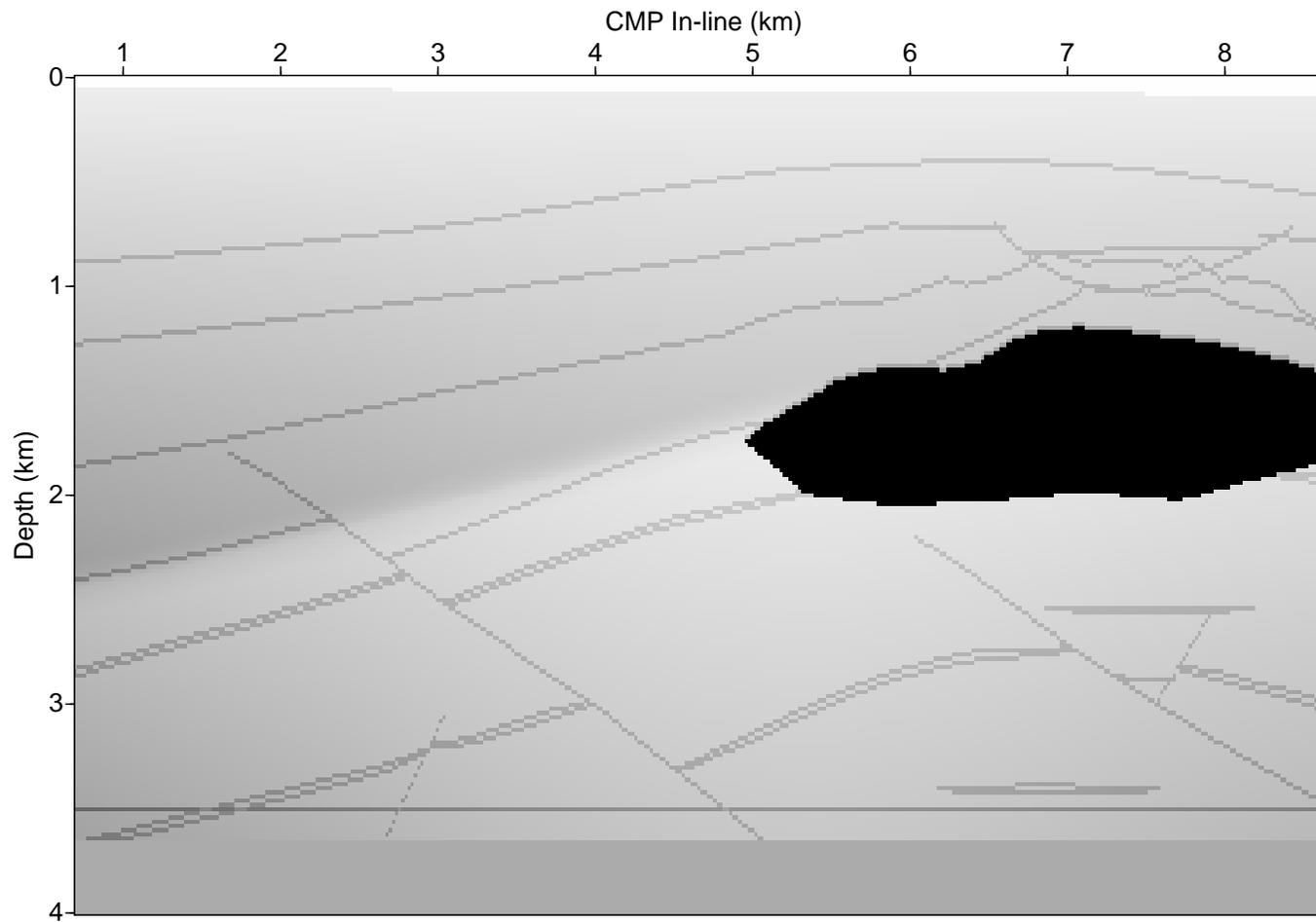
SEG-EAGE salt model: in-line section at constant cross-line coordinate  $y = 9,820\text{m}$ .
