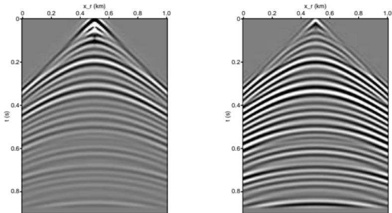
Left: Simulated seismic response of rough model ( $\mathcal{F}[0.95v + r]$ ),
