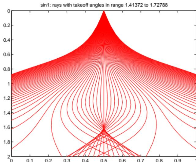
Rays in sinusoidal velocity field, source point = origin. Note formation of caustic, multiple rays to source point in lower center.
