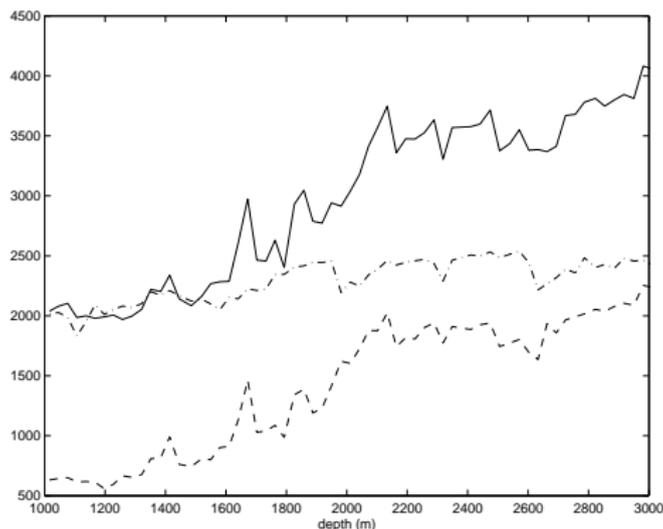
Blocked logs from well in North Sea (thanks: Mobil R & D). Solid: p-wave velocity (m/s), dashed: s-wave velocity (m/s), dash-dot: density (kg/m<sup>3</sup>). “Blocked” means “averaged” (over 30 m windows). Original sample rate of log tool < 1 m.
