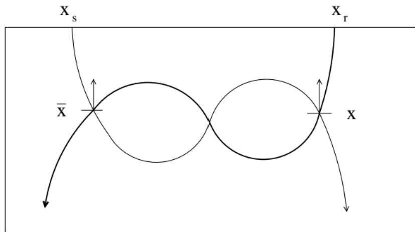
Symmetric waveguide: time ( $x_s \rightarrow \bar{x} \rightarrow x_r$ ) same as time ( $x_s \rightarrow x \rightarrow x_r$ ), so TIC fails.
