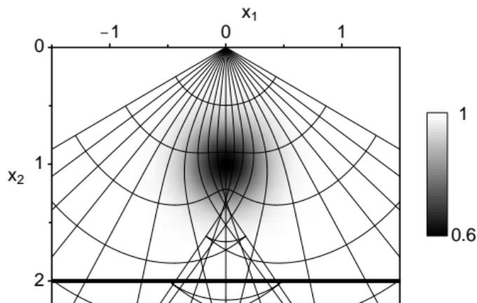
Gaussian lens velocity model, flat reflector at depth 2 km, overlain with rays and wavefronts (Stolk & S. 2002 SEG).
