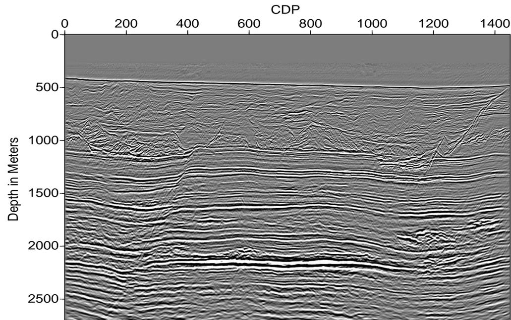
Example of GRT Inversion (application of  $F[v]^\dagger$ ): K. Araya (1995), “2.5D” inversion of marine streamer data from Gulf of Mexico: 500 source positions, 120 receiver channels, 750 Mb.
