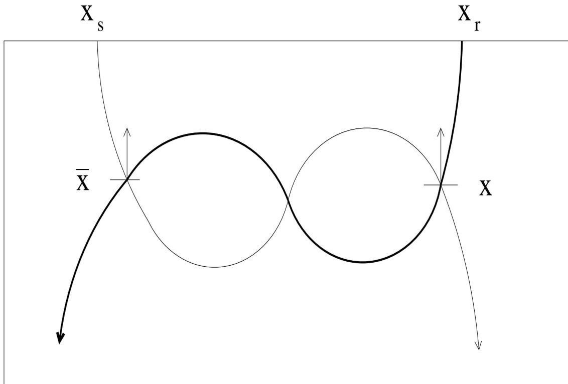
Symmetric waveguide: time ( $x_s \rightarrow \bar{x} \rightarrow x_r$ ) same as time ( $x_s \rightarrow x \rightarrow x_r$ ), so TIC fails.
