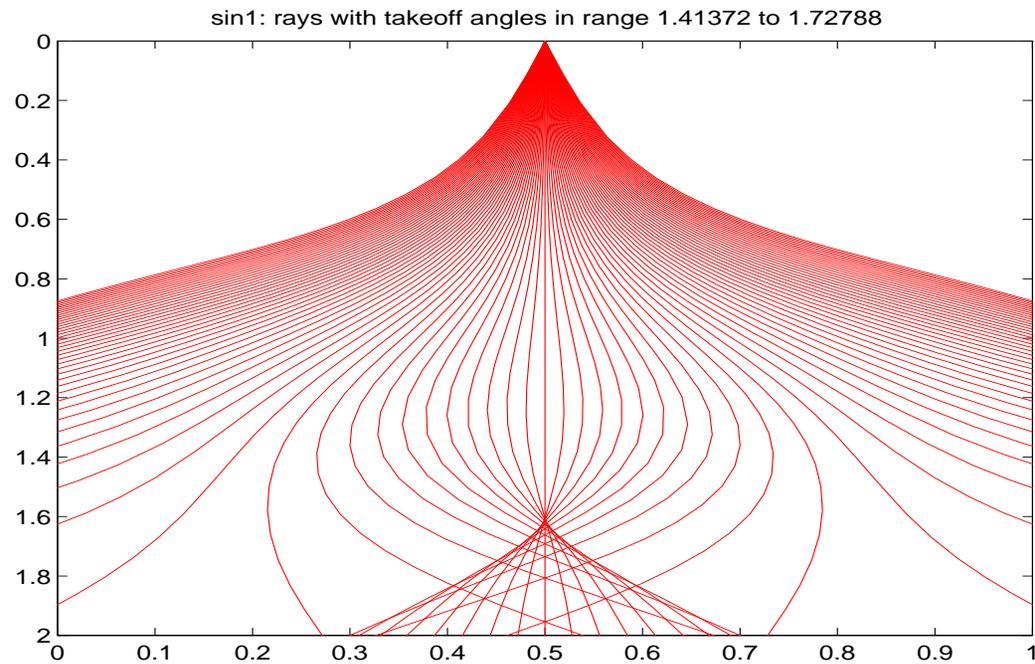
Rays in sinusoidal velocity field, source point = origin. Note formation of caustic, multiple rays to source point in lower center.
