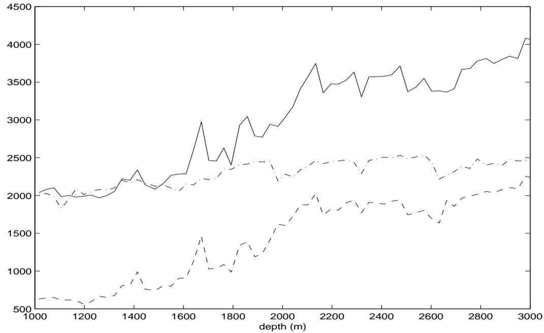
Blocked logs from well in North Sea (thanks: Mobil R & D). Solid: p-wave velocity (m/s), dashed: s-wave velocity (m/s), dash-dot: density (kg/m<sup>3</sup>). “Blocked” means “averaged” (over 30 m windows). Original sample rate of log tool < 1 m. **Reflectors** = jumps in velocities, density, **velocity trends**.
