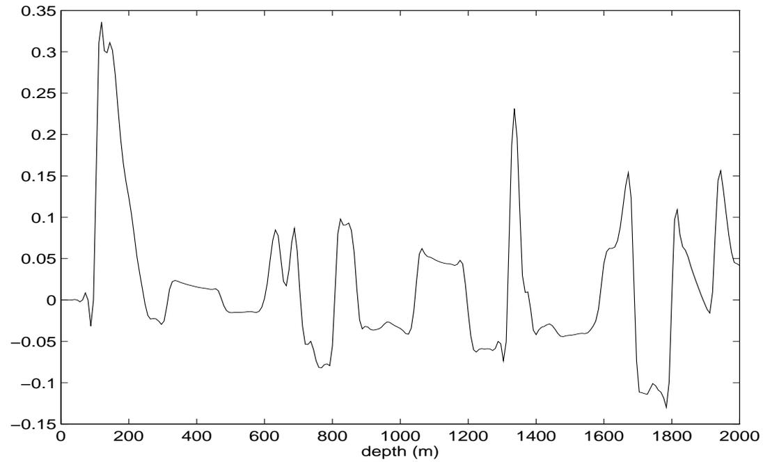
Reflectivity function  $r(x_1)$  (function of depth only) used in numerical linearization study.
