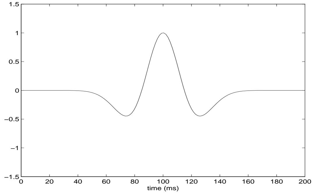
Source pulse  $w(t)$  used in numerical linearization study.
