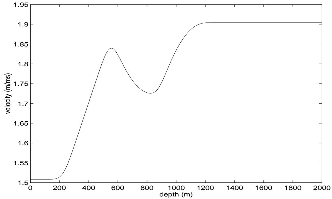
Velocity  $v(x_1)$  (function of depth only) used in numerical linearization study.
