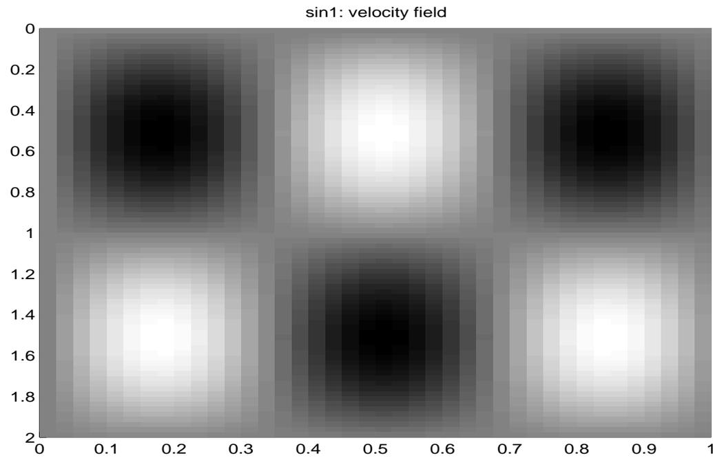
2D Example of strong refraction: Sinusoidal velocity field  $v(x, z) = 1 + 0.2 \sin \frac{\pi z}{2} \sin 3\pi x$
