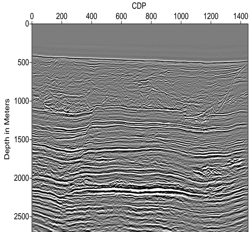
Example of GRT Inversion (application of  $F[v]^\dagger$ ): K. Araya (1995), “2.5D” inversion of marine streamer data from Gulf of Mexico: 500 source positions, 120 receiver channels, 750 Mb.
