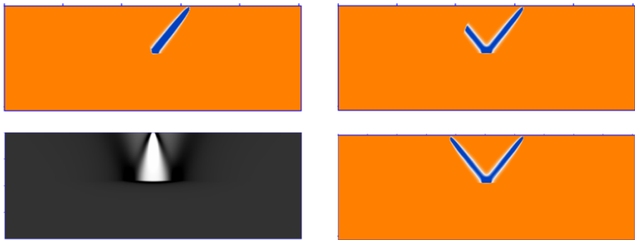
Figure : Partial gradient images at times t=0.87s , 0.39s , respectively for the top two plots (in clockwise). The bottom right plot corresponds to the final complete gradient corresponding to this trace, i.e., at time t=0.0s . The bottom left plot is the gradient after an inversion of a shot gather.
